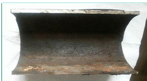
Figure 1. The corrosion characteristics of the oil collecting pipeline under the scale are obvious
