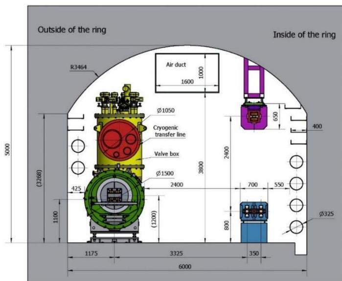
Figure 3. [6] Cross section of the tunnel
