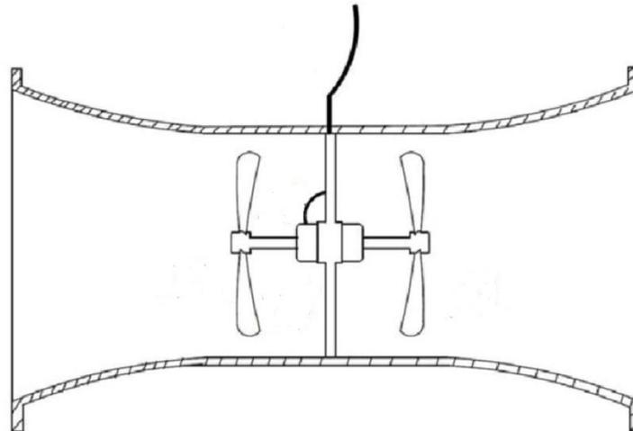
**Figure 1.** Sectional view of water flow generator
