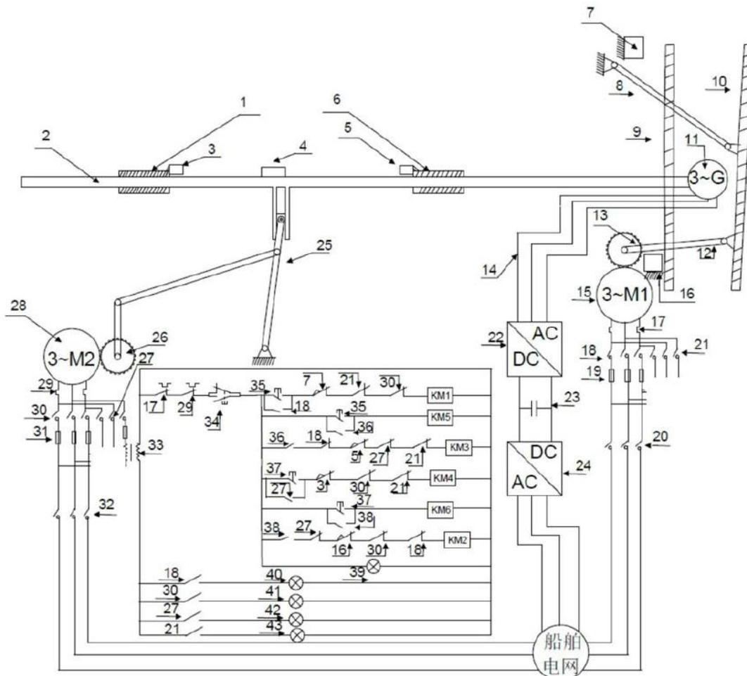
Figure 2. Schematic diagram of water flow generator expansion.
