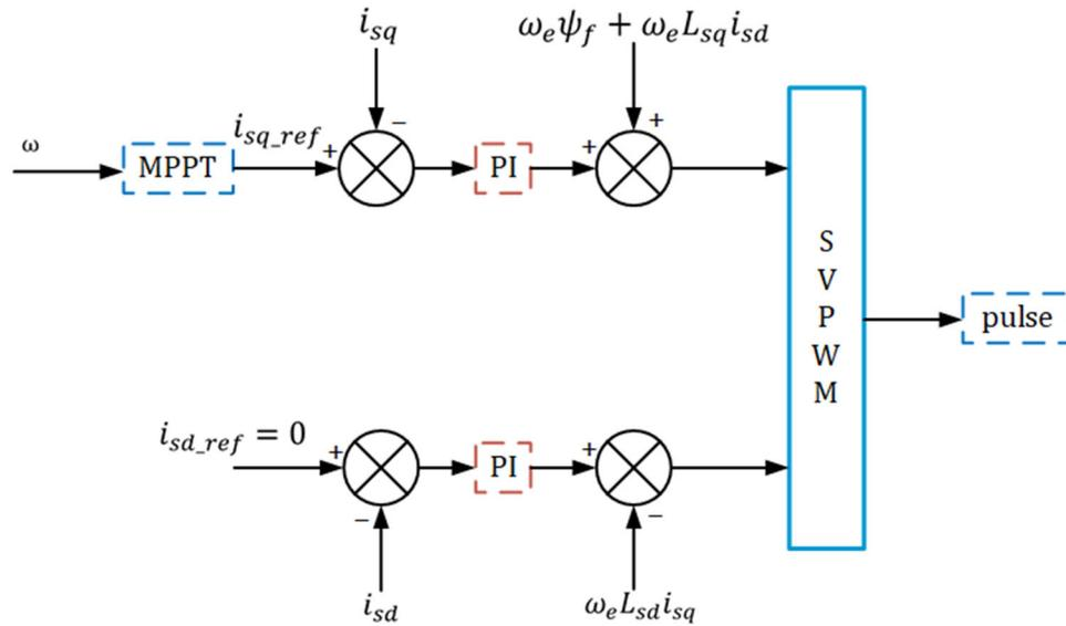
Figure 2. Control block diagram of generator-side converter
