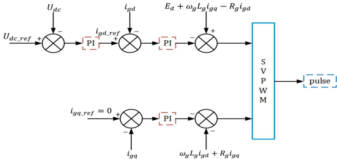
Figure 3. Control block diagram of grid-side converter
