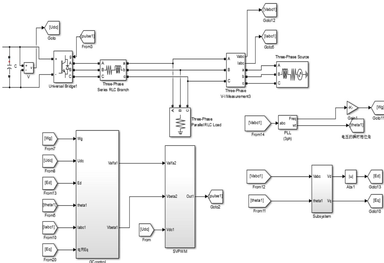
Figure.10 The simulation model of grid side
