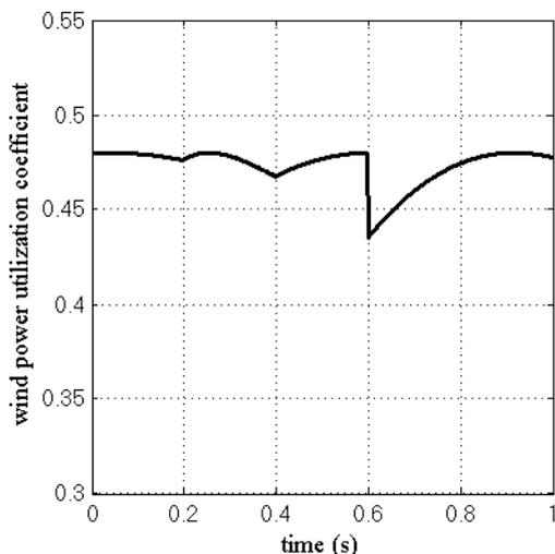
Figure 6. Wind performance coefficient
