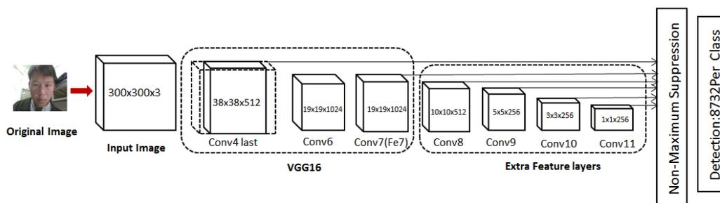
Figure 1. SSD Network Structure Diagram
