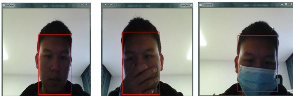
Figure 4. Detection result of face detector
