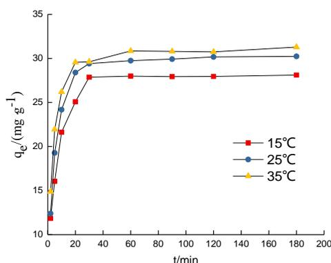
Fig.1 Adsorption equilibrium curve of  $\text{Cd}^{2+}$  by modified rice dusks
