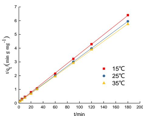
Fig.3 Pseudo-second equation of Cd<sup>2+</sup> adsorption by modified rice husk
