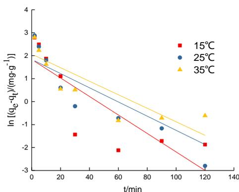
Fig.2 Pseudo-first equation of Cd<sup>2+</sup> adsorption by modified rice husk
