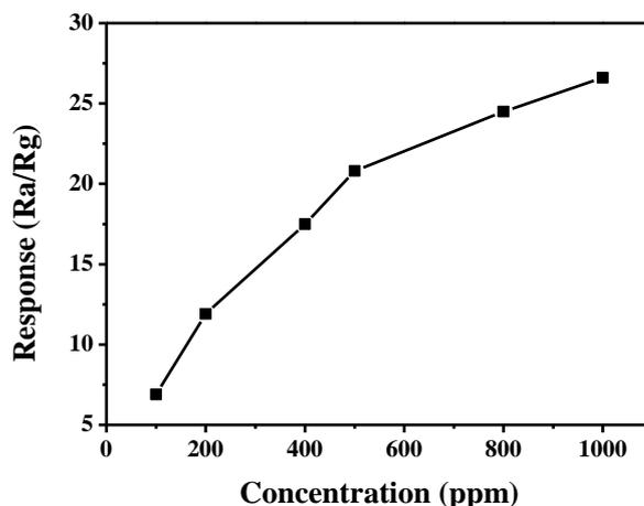
Fig. 3 Responses of the ZnSnO<sub>3</sub> sensor to different concentration ethanol at 400°C
