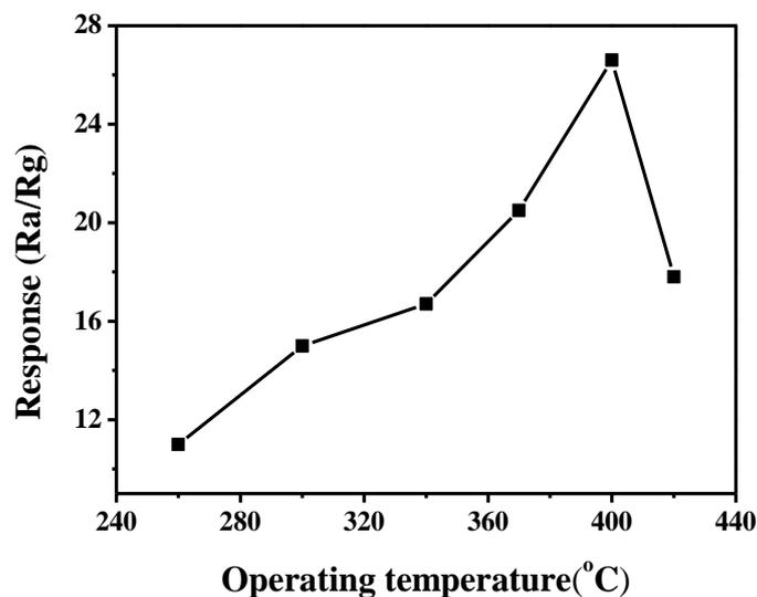
Fig.2 Responses of the ZnSnO<sub>3</sub> sensor to 1000 ppm ethanol at different temperature
