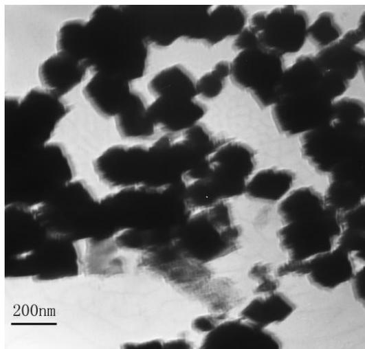
Fig. 1 TEM photographs of ZnSnO<sub>3</sub> nanoparticles
