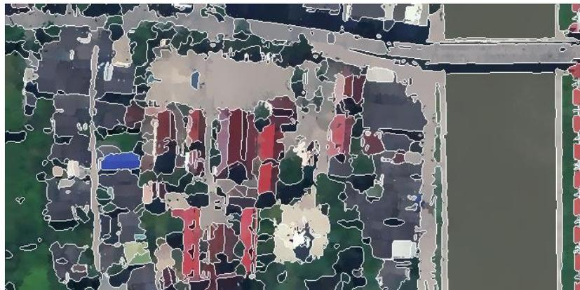
Fig. 3 MS mean drift processing results graph
