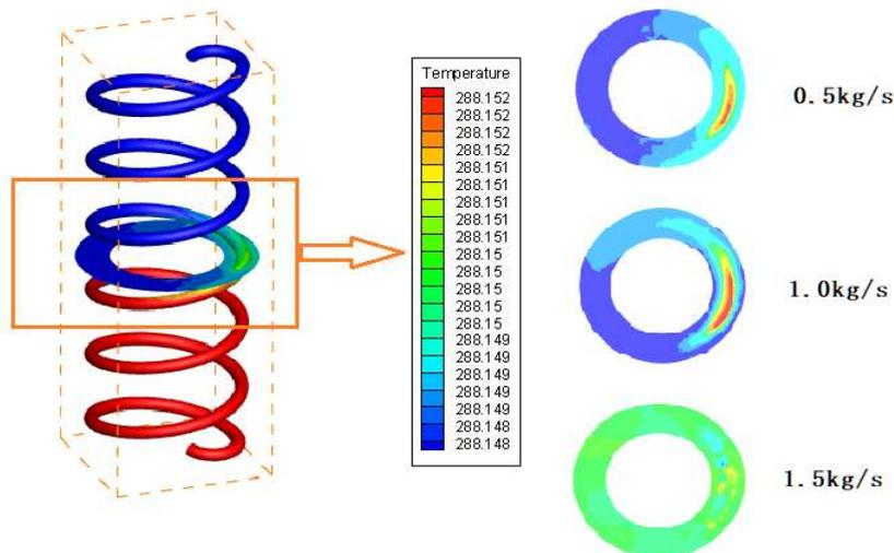
**Figure 7.** Temperature cloud diagram (cross section) under different cooling air flow
