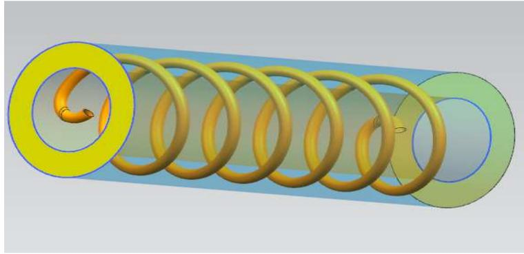
**Figure 1.** Spiral tube heat exchanger model
