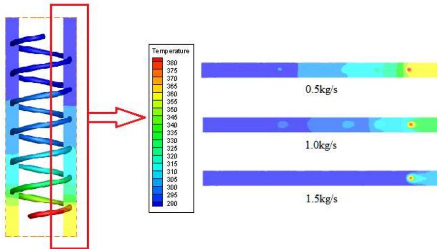
**Figure 6.** Temperature cloud diagram under different cooling air flow (longitudinal section)
