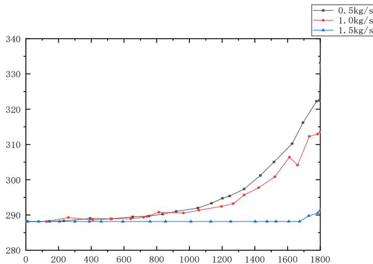
Figure 8. Broken line diagram of cooling fluid temperature under different inlet flow
